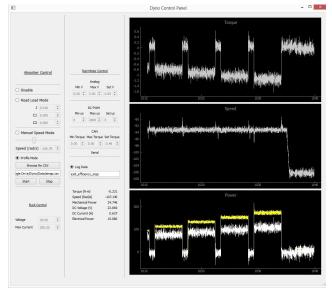
Figure 2: Dyno Software control panel mid-experiment
