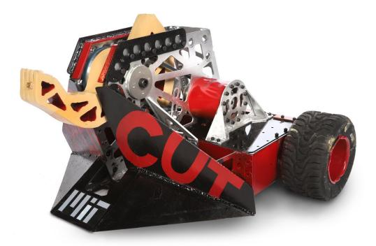
Uppercut sports a 50lb vertically spinning fist shaped blade. The fist spins at around 3000 rpm, giving us an effective tip speed of around 200mph. It's made of AR500 (abrasion resistant steel) and packs quite a punch.
