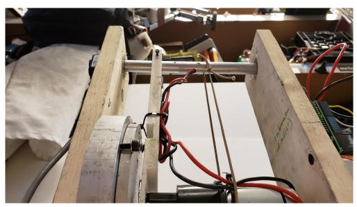
A fun closeup shot of the neat trick for attaching the inertial rim to the wheel, and how barely the new motor + flywheel fit in between the wooden posts.
