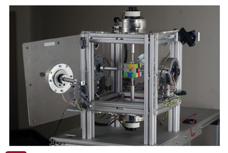
To fix this, we tightened all the faces. This made the cube much stiffer, and harder to solve by hand, but it ended up being better for the machine. To increase the lifetime of the cubes, we added some grease to the screws. Even then, they still occasionally exploded.
