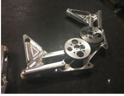
Gripper machined assembly
