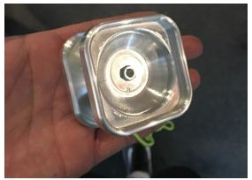
The First Protoype was made on MITERS CNC mill and manual Bridgeport
